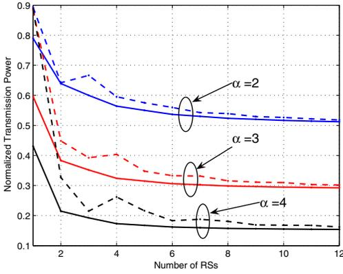
Fig. 3. Normalized transmission power. Dashed lines correspond to evenly placed RSs, while solid lines correspond to the optimal placement.
