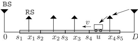
Fig. 1. One-dimensional highway cellular network with  $M = 4$  RSs between two BSs. A vehicle at position  $u$  is traveling with speed  $v$ , served by two-hop DF relaying. Each rectangular box represents the coverage of an RS.
