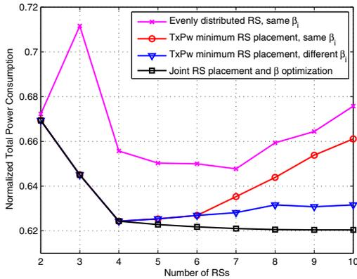
Fig. 4. Normalized total power consumption with  $\alpha = 2$ .
