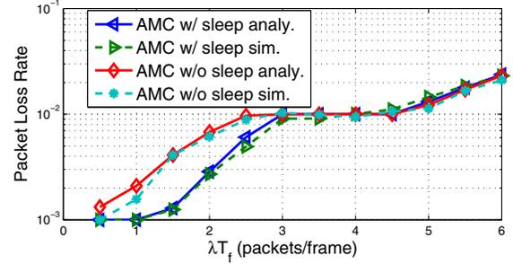
Fig. 4. Packet loss rate of AMC with sleep and without sleep.
