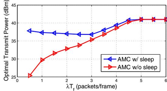
Fig. 3. Optimal transmit power of AMC with sleep and without sleep.
