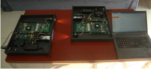
Fig. 2. bi-directional VLC system entities between the train and the station.
